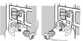
2) Loosen the cylinder lock wing nut. Swing the cylinder lock down. Tighten the wing nut.
